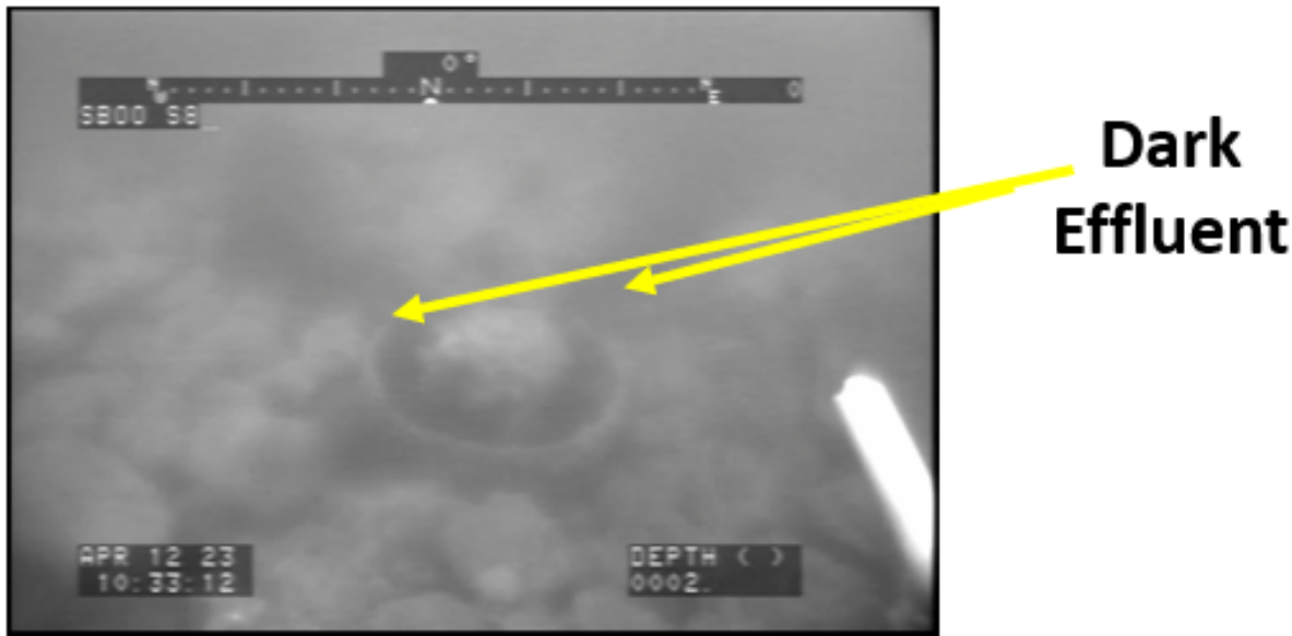
Figure 19 Picture from the City of San Diego's inspection of SBOO outlets on April 12, 2023, that displays the atypical effluent discharge darker than the normal effluent pictured in Figure 18.
