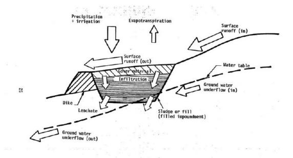
Figure 3-1. Simplified Water Balance for Filled Surface Impoundment
