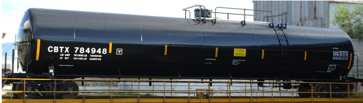
Figure 77: 33,700 Gallon Pressure Tank Car 175
