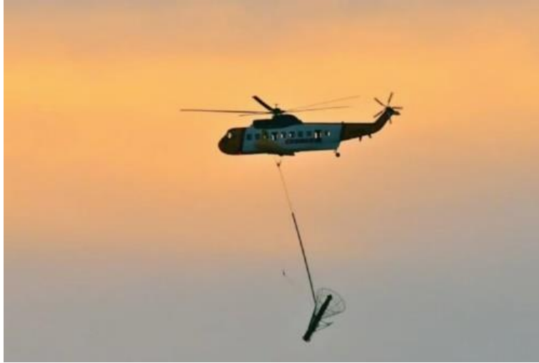
A Croman SIKORSKY S-61N Helicopter with a Torpedo in Its Recovery Basket
