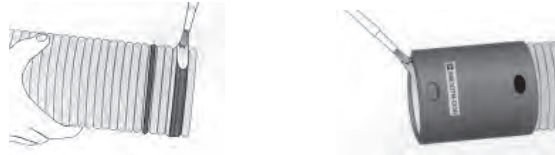
Figure 25 Key-Lock™ Couplers Lubricant Application
