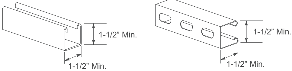
Figure 10 Typical Strut Channels Used for Panel Board Construction
