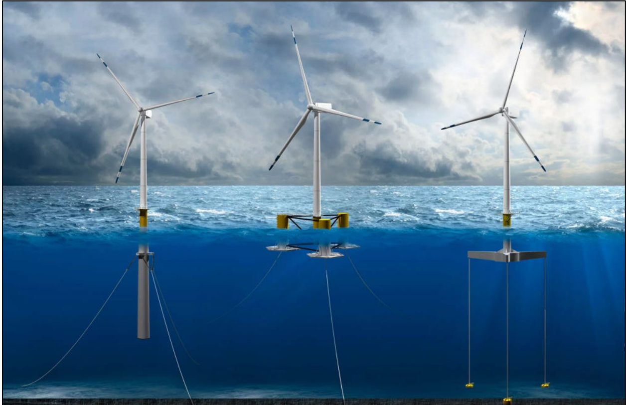
Figure 3. Illustration of floating foundation types (left to right: spar, semi-submersible, TLP) (NREL 2022)
