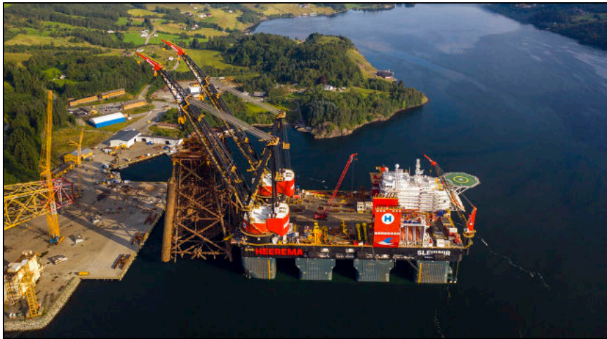
Figure 20. Sleipnir loading Brent Alpha’s upper jacket onto the wharf at AFOD Facility in Norway (Heerema Marine Contractors)
