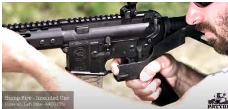
Figure 2: After the first shot, the shooter's finger rests against the extension ledge of the bump stock, which "constrains" the recoil and the opposing forward force so that the firing unit slides in a linear direction, propelling the firing unit against the stationary finger, causing the firing cycle to repeat.
