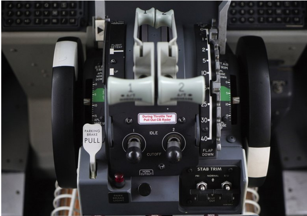
Center console of 737 MAX, with manual stabilizer trim wheels at left and right. Cut-out switches are at lower right.
