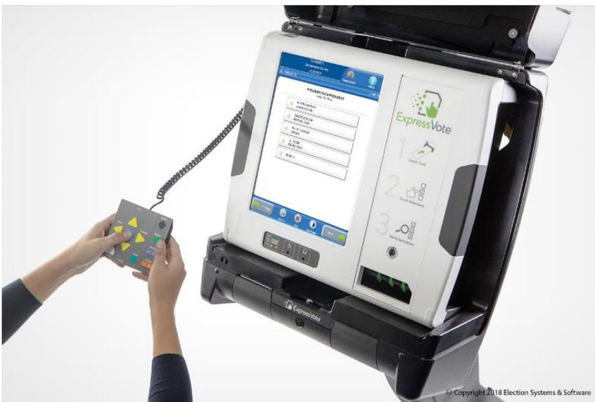
52. To use the ExpressVote, the voter inserts a piece of blank thermal paper to activate the machine. The voter may use the touch screen or audio-tactile keypad to make selections.
