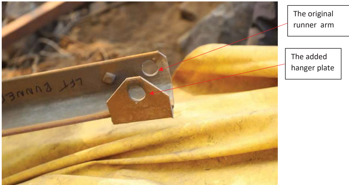
Figure 6. The left runner arm and the added hanger plate from the Incident Tower. 82
