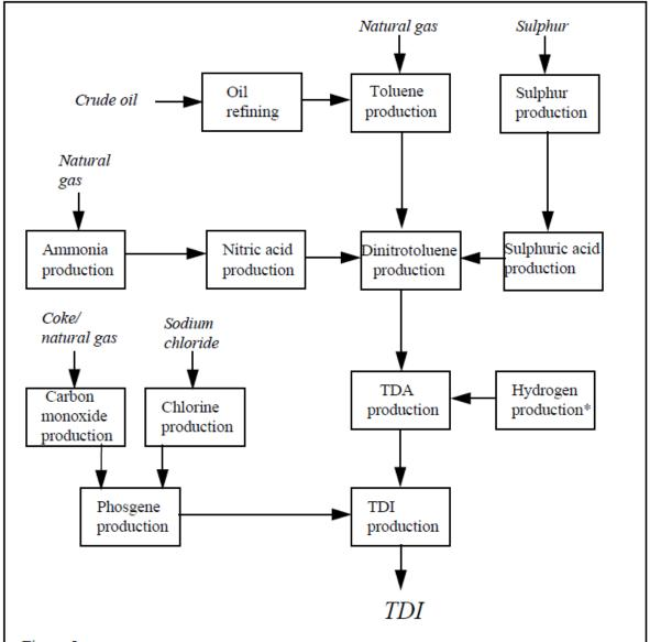
Schematic diagram showing the principal operations leading to the production of TDI.
