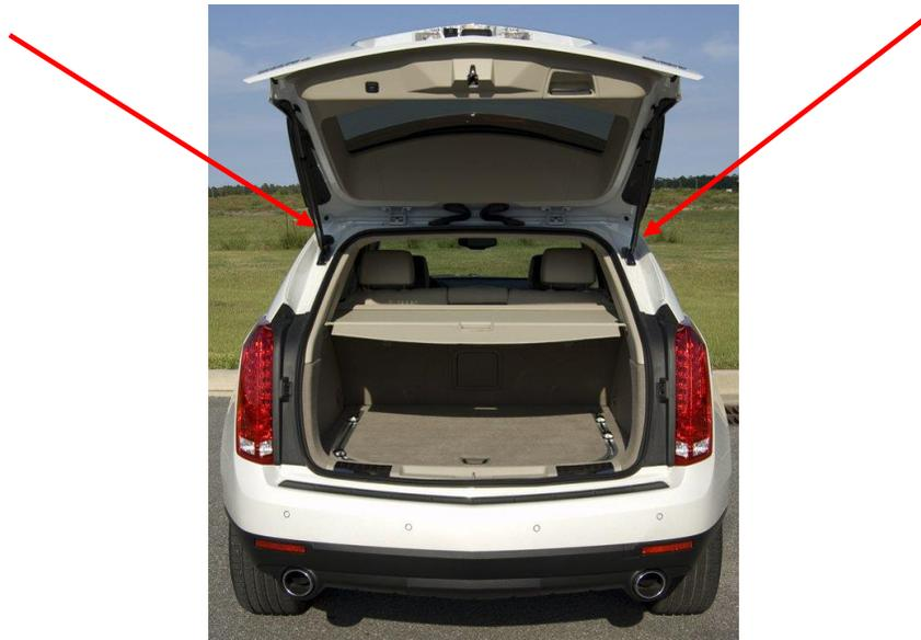
39. Inside each strut is a piston rod that slides in and out of the cylinder, which is sealed at the top to retain pressurized nitrogen gas inside. The stored gas provides the pressure to hold the heavy rear liftgate in the open position. In order to hold the liftgate, the cylinder seal has to prevent the gas from escaping.
