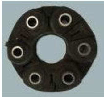
6. A triangular flange connecting the flex disc to the transmission is bolted on to one side of the flex disc using three of the holes; a similar triangular flange connecting the flex disc to the driveshaft is bolted on to the other side of the flex disc using the other three holes.
